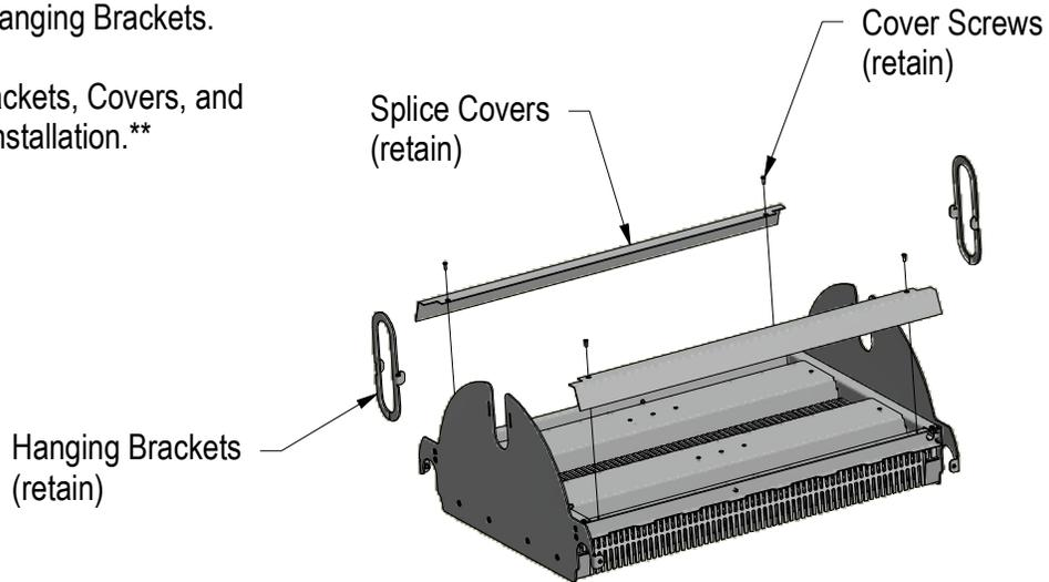
**STEP 2:** Dismantle Existing Fixture Unit. Remove Lamp, Ballast, and any Covers to exposed Supply Leads. Cut Supply Leads.
